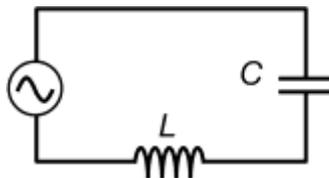
Connect the inductor and capacitor in series with the signal generator. Place the AC voltmeter in parallel with the capacitor, so that you measure the rms voltage  $V_{Lrms}$  across it. Scan the frequency of the signal generator to find the frequency giving the maximum
