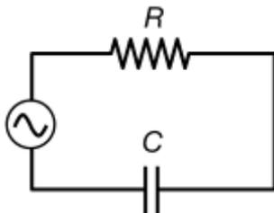
Use only dielectric capacitors. Do not use an electrolytic capacitor, as they are ruined by currents of the wrong polarity.
