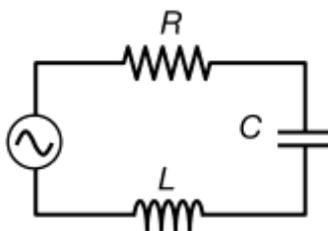
Now add some resistance to the circuit (in addition to the intrinsic resistance of the inductor) by placing a resistor in series with the inductor and capacitor. Again, find the resonant frequency of the circuit by adjusting the source frequency to give the greatest  $V_C$  or  $V_L$ . Use three different resistances, one near the characteristic resistance  $R_0 = \sqrt{L/C}$  and the other two below it. Fill in the remaining columns of the tables. Calculate  $I_{rms}$  as  $V_{Rrms}/R$ .
