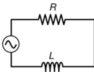
First, use the ohmmeter to measure the resistance  $R_L$  of the inductor as if it were a resistor and record it below. Place the inductor in series with a resistor and the signal generator. Investigate the circuit using sine waves at the indicated source frequencies. At each frequency, find a resistor (resistance  $R$ ) that gives  $V_{Rrms} \approx V_{Lrms}$ . Record the measured values of  $R$ ,  $V_{rms}$ ,  $V_{Rrms}$ , and  $V_{Lrms}$ .
