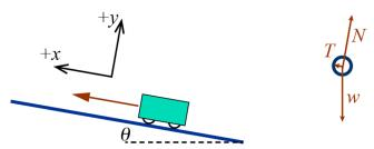
In this problem there is an incline but no friction. The car will move along the incline, so it will be most convenient to use inclined coordinates, tilted by ten degrees. The components of the car's weight mg = (1720 kg)(9.8 N/kg) = 16856 N are  $w_x = -w \sin \theta = -2927 \text{ N}$  and  $w_y = -w \cos \theta = -16600 \text{ N}$ .
