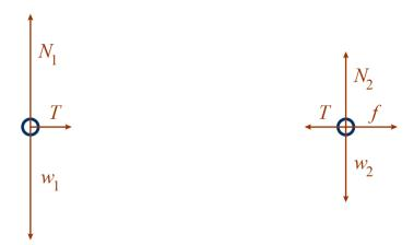
The greatest force that can pull the drive cart forward is friction between its wheels and the track,  $f = \mu m_2 g$ . The track is level, so the normal forces exactly cancel each car's weight. Tension in the cord between the carts pulls the pulled cart forward and the drive cart backward. Because the cord links the carts, their velocities and accelerations are the same.
