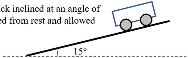
The constraint imposed by the normal force on the cart is that the cart will not accelerate normal to the track. Find the acceleration of the cart. (I suggest using a components table.)
